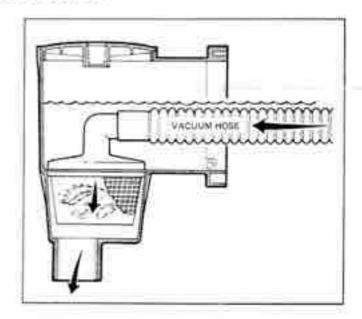
NOTE: Take care not to damage or scuff up SKIM-VAC's specially designed sealing surface.
